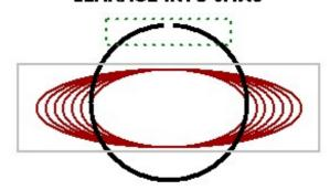
Wrap Round Coil Design where jaw opening is inside the coils field gives potential for magnetic flux leakage increasing reading errors.
